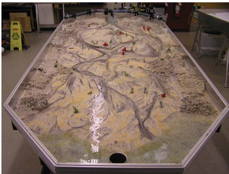
(a) A stream of water flowing over sand can simulate the evolution of a river.
